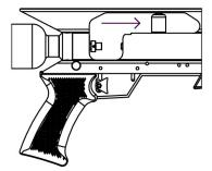
Cock the pistol by pushing forward on the cocking knob until the bolt clicks and stays open like this. the safety has also set automatically. You can now load one pellet into the back of the barrel, making sure to push it as far into the barrel as possible.
